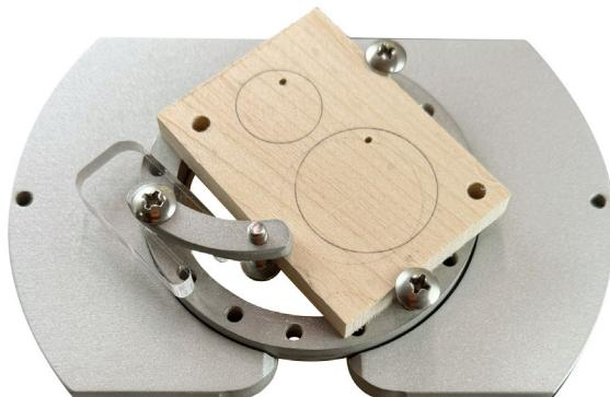
Use the Slider Supports under screws to hold thicker material with the WorkFingers.
