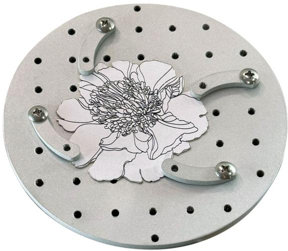
WorkFingers and Slider Supports can be used as clamps when holes are not in correct alignment to be screwed into directly. Use the slot to move the Slider Support into position, then screw into the WorkDisc. Either end can be used as a clamp.
