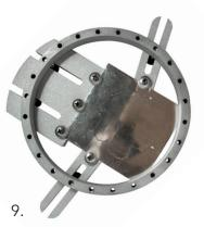
10. Use thin rulers or thin strips of metal on top of and underneath partially sawed metal for support. This will keep it from moving up and down as you saw.
