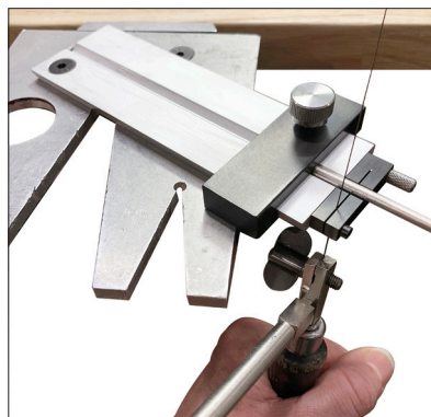
Sawing left handed. Jig mounted on the Jayne Redman® Rotational Bench Pin.
