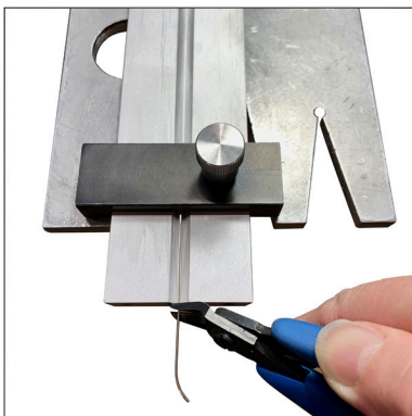
Remove the saw guide to flush cut wire.
