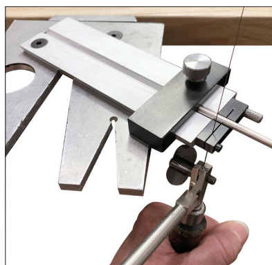
Sawing left handed. Jig mounted on Jayne Redman® Rotational Bench Pin for hands free use.
